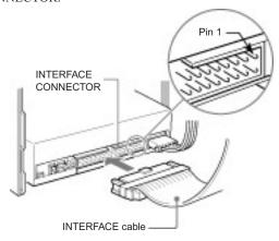
**2** Attach the other end of the cable to the PRIMARY or SECONDARY IDE interface connectors on the computers mainboard.
